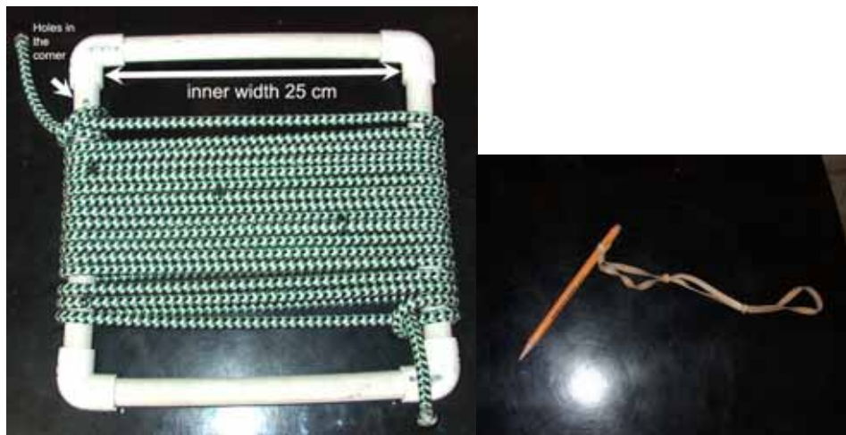
(c) Details of the quadrat: note the holes on the corners to let the air and water out, example of the rubber band leash for rulers and pencils (If available, we recommend PaperMate® Sharpwriter mechanical pencils).
